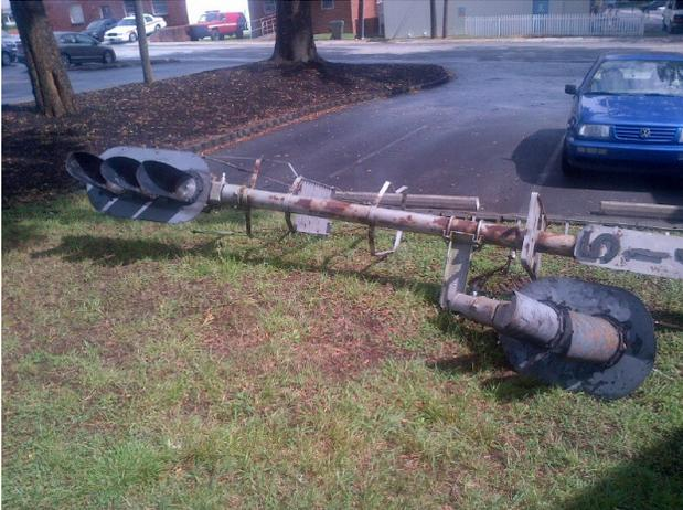
The lower head bracket appears to be broken as the head is not connected to the bracket. Maybe it was damaged in transit. I don't know where the second signal is hiding. I reckon the city has it someplace.
