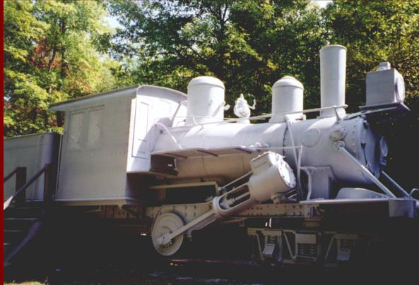
A Climax locomotive is a type of geared steam locomotive in which the two steam cylinders are attached to a transmission located under the center of the boiler. This transmits power to driveshafts running to the front and rear trucks.
