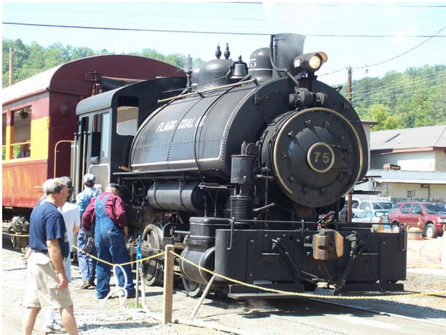
Flagg Coal Company #7, an 0-4-0 saddle tank steam locomotive at Bryson City in September 2007.
